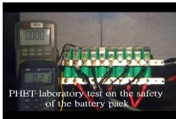
Figure 6 Photographic picture of a DOSBAS® battery system assembled with cells in C- \text{LiFePO}_4 chemistry being short-circuit tested with no increase in cell temperature and visible cell damage except the blown fuses.
