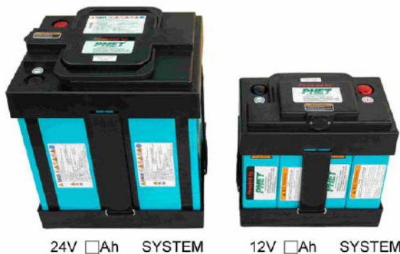
Figure 8 Photographic picture of two battery packs assembled for 12V and 24V applications embedded with the DOSBAS ® system and voltage balancing boards on top of the packs.
