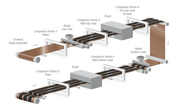
End-to-end coating process monitored and controlled at all stages
