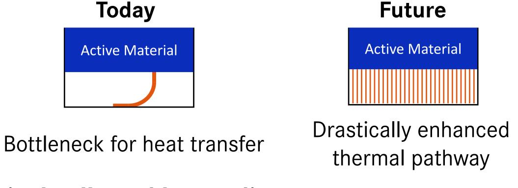
New possibilities for future automotive battery pack design with tabless cylindrical cells and larger diameters
